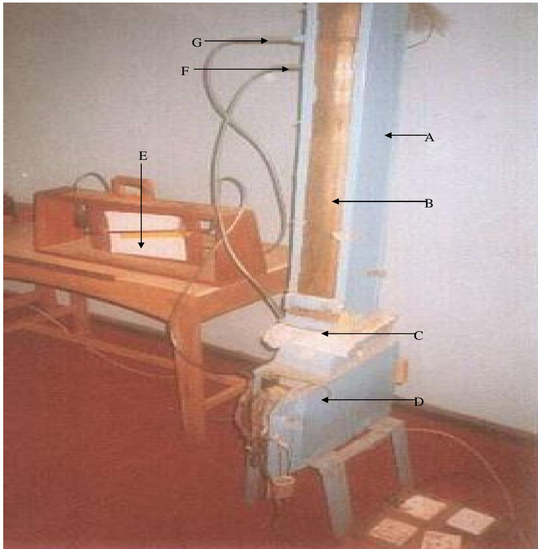
**Figure 2: Terminal Velocity Test Equipment**
