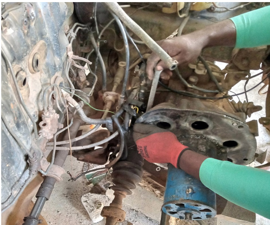
Figure 4: Coupling of DC Motor and Adapter Plate with the transmission of the donor car
