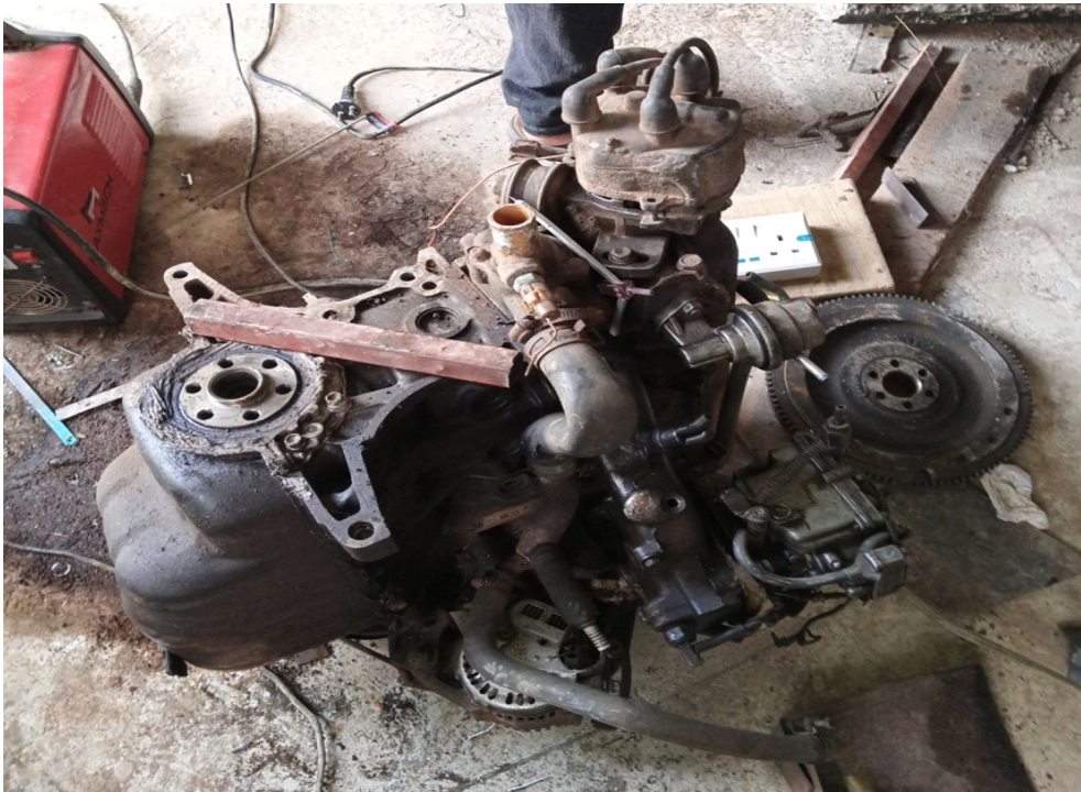
Figure. 1: ICE removed from the Toyota Starlet Car
