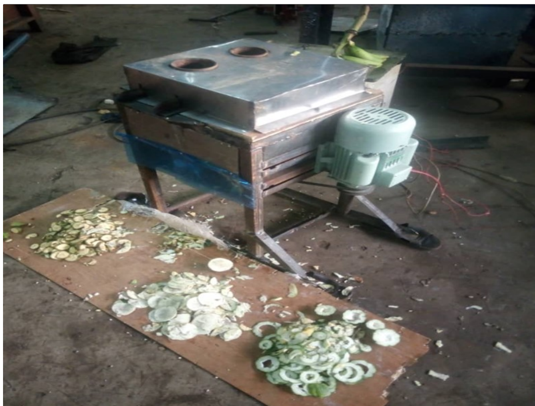
Figure 7: Developed two-way slicing machine
