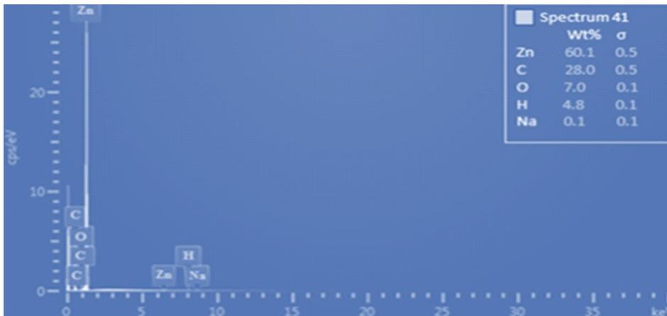
Figure 3: EDS Spectra of the Coatings (Sample P8)
