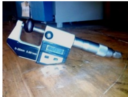
Plate 1: Size determination by micrometer screw gauge
