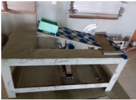
Plate 2: Angle of repose apparatus
