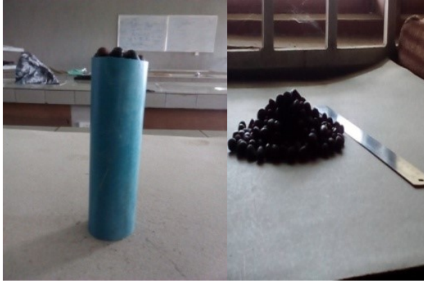
Plate 3: Determination of angle of repose
