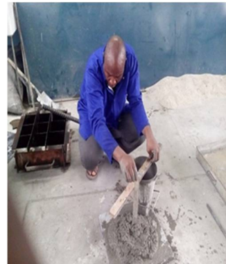
(c) collapsed slump
