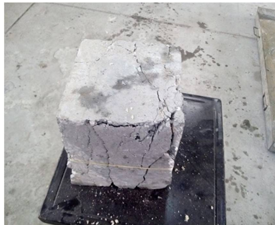
Plate2b: Failure Pattern
