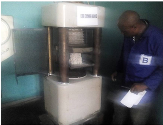
Plate 2a: Failure Mode of Concrete Cube.
