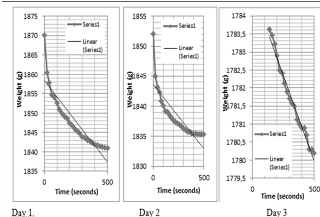
**Figure 6: Drying curves for the different days of the experiment.**
