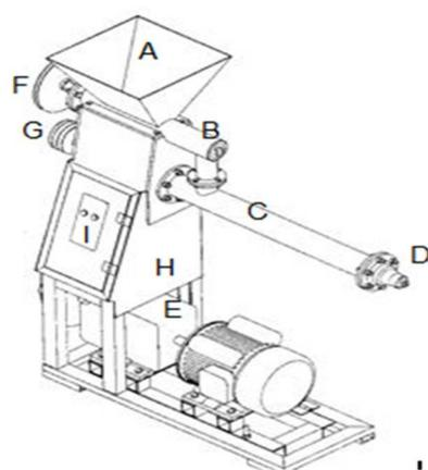
Figure 1: Isometric drawing of the extruder used- LEGEND A- Hopper, B- Feeding Conveyor, C- Extruder worm, D- Die Unit, E- Power train, F- Conveyor pulley, G- Extruder pulley, H-Extruder Housing, I- Control switch
