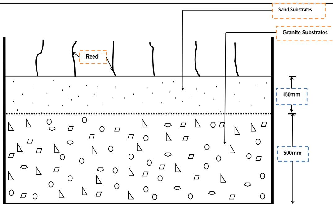
**Fig. 3: Section through the CW showing the various components of the CW system**
