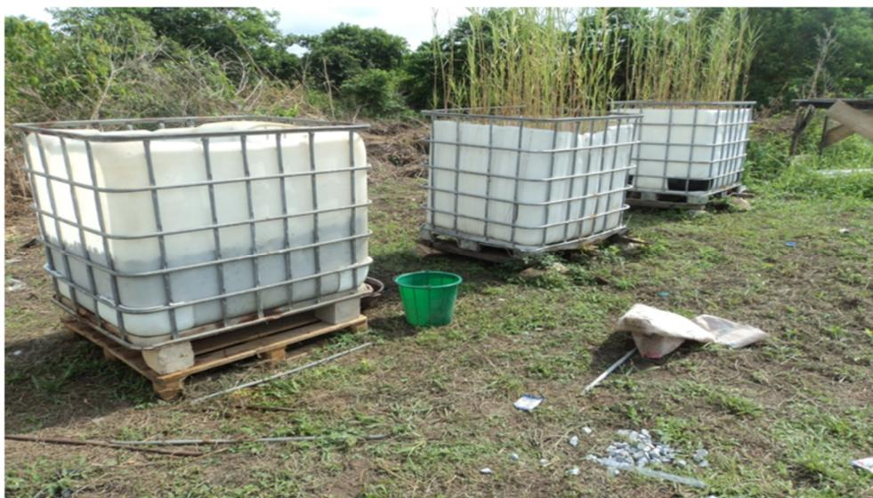
Fig. 2: Setup of the pilot scale CW at Umar Kabir Hall, Federal University of Agriculture, Abeokuta, Nigeria
