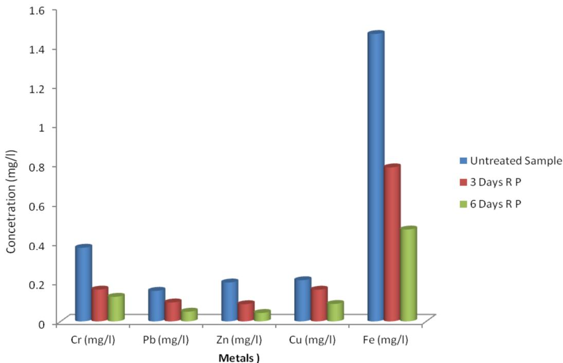
**Fig. 4: Reduction in heavy metals with change in retention period in Pilot Scale CW**
