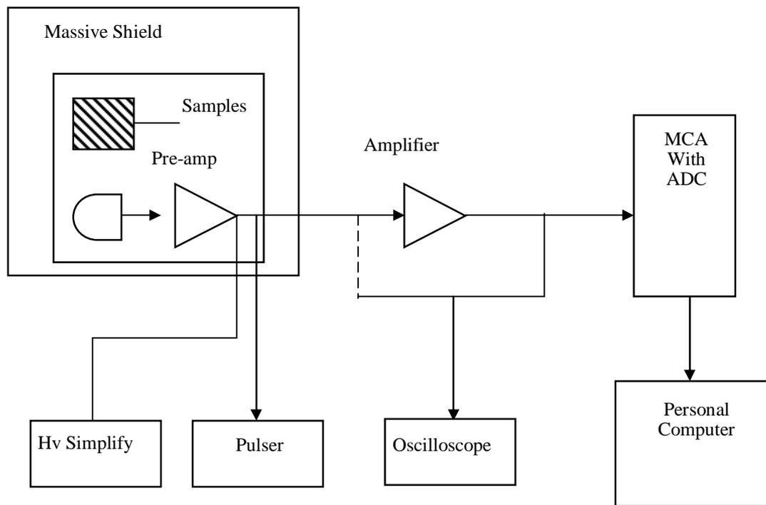
Figure 1. Schematic diagram of the detector, high purity germanium crystal
