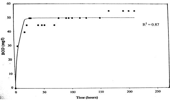
Figure 3: Effect of 125mg/l on BOD at 20°C
