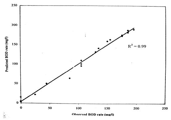
Figure 8: Scatter plot of the predicted versus observed BOD rate at 40°C and lead concentrations of 50mg/1
