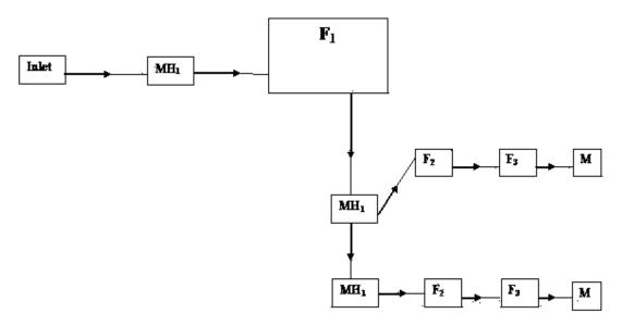
Figure 1: Schematic diagram of the waste stabilization ponds at the University of Dar-es-Salaam
