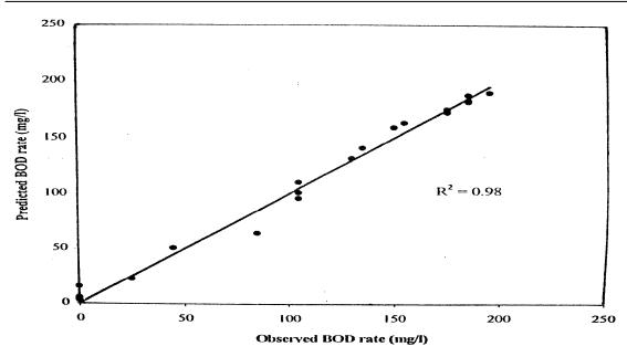
Figure 7: Scatter plot of the predicted versus observed BOD rate at 35°C and lead concentrations of 50mg/1
