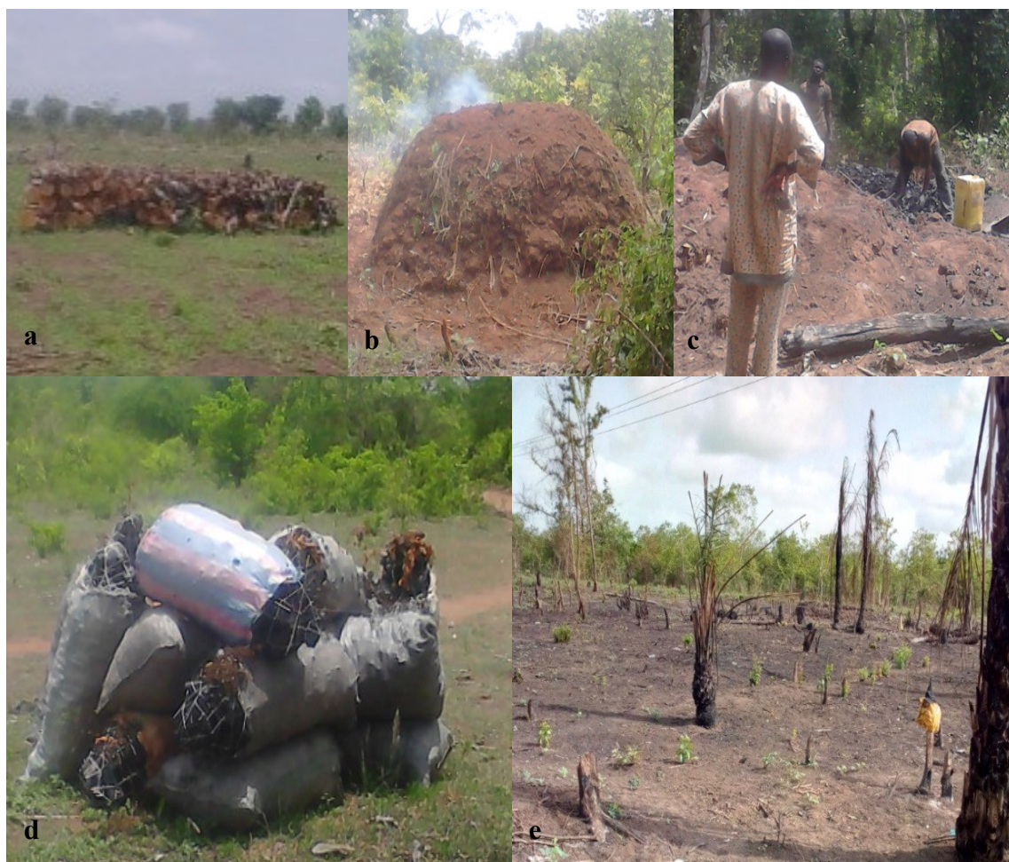
Figure 2: Traditional earth mound kiln method of charcoal production process in the study area
