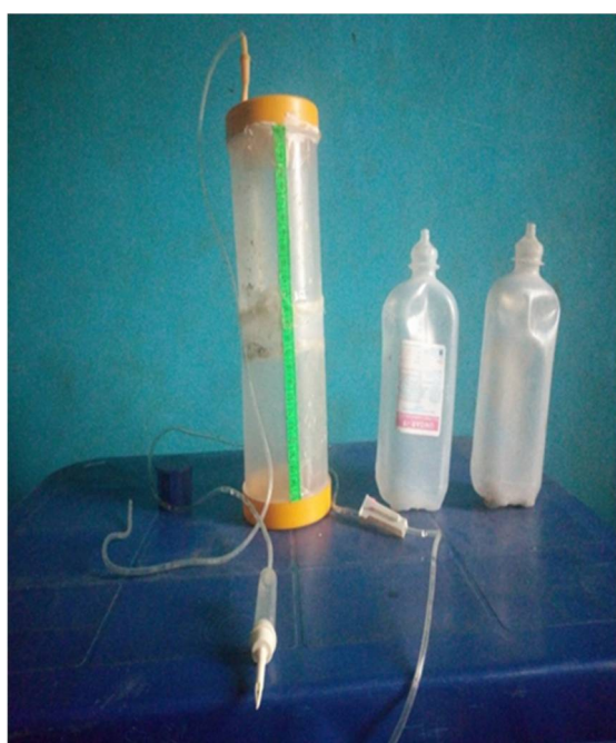
Figure 2: An improvised calibrated permeameter and schematic arrangement Procedures for permeameter usage
